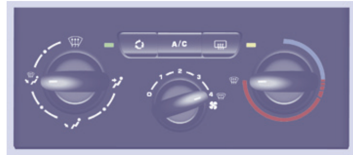
Air conditioning control panel
