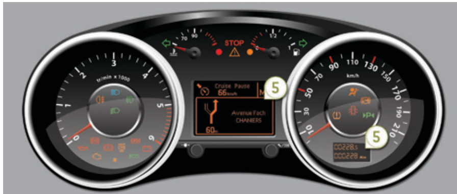
Panel grouping together the vehicle operation indication dials and warning lamps.
